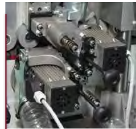
Automatic chain feeding milling and bending machine
